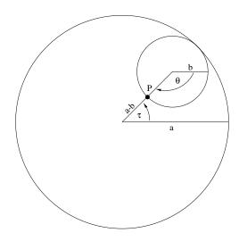
inner circle have a radius b. After the inner circle has rotated through an angle  $\theta$ , the center of the inner circle has rotated through an angle  $\tau$ . If the inner circle rolls without slipping, then  $b\theta = (a - b)\tau$ . The coordinates of a point P on the inner circle are then
